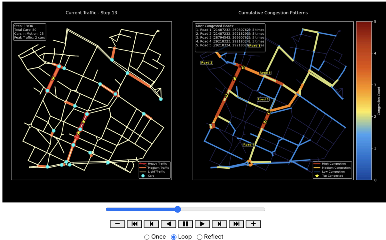
Figure 3. While Figure 2 showed a strong static snapshot of congestion, I wanted to better illustrate how congestion develops over time, so I created an animation with 30 frames (see Cell 6). Each frame shows live traffic (left) and cumulative congestion (right) as cars move through the network. The left side updates dynamically with car positions, traffic levels (color-coded), and intersections marked red when overloaded. The right side builds up a congestion count – roads turn from blue to red based on how often they were congested. In this case, a road is marked “congested” if the number of cars trying to enter it exceeds 50% of the peak traffic in that step. This dual view makes it easier to see both short-term traffic jams and long-term structural bottlenecks.
